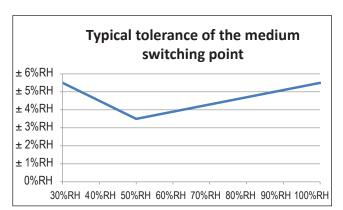
1-point-adjustment at 48 % RH/23 °C Long-term drift: ≤ ± 1 % RH p.a.
