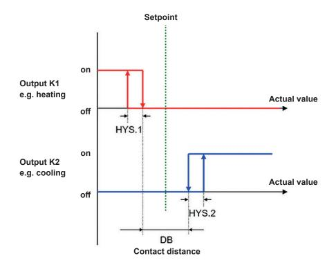
The setpoint is always in the centre of the contact distance. When the setpoint is changed, the entire curve moves along with the setpoint.
